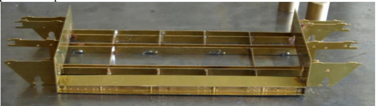
There is a honeycomb of small parts that go to make up the bed of the vehicle before the deck is fitted, which I soldered in after the end plates had been fitted.
