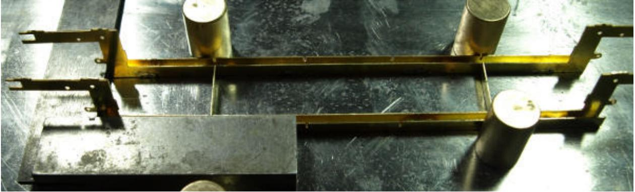
The central frames need careful attention, especially when constructing the channels, which are basically edge soldered though there some tabs and half slots to help.
