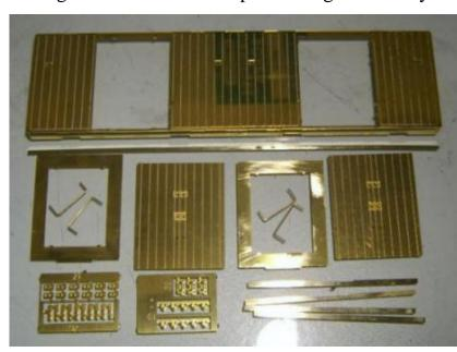
drawing and the parts is essential but, once figured out, is not difficult. The long folds on each side, and especially the solebars, were done using my newly acquired "Hold & Fold". This excellent tool has enabled me to make 1 and 2mm folds over long sections perfectly straight and at right angles with no cockling.
