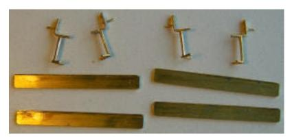
The steps, which fit under the doors, are intended to be fitted using wire and etched supports. The method works well but I prefer to use Slater's
