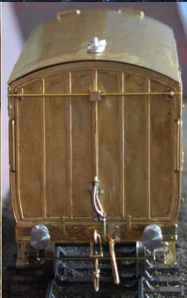
Here is a shot of an end with Westinghouse brake now fitted.
