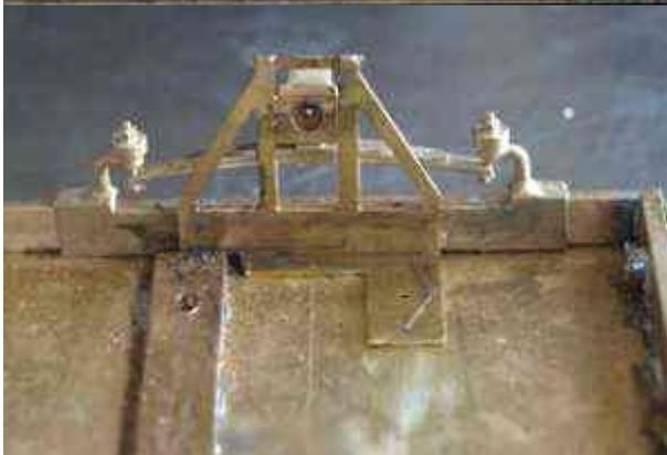
A set of spare W irons from a Slater's Cleminson underframe were suitably modified and soldered in behind the CPL long J hanger springs. These can better be seen in the next two pictures. The axle box is soldered to the W iron. The integral, sprung buffers were liberated from a Slater's Dean clerestory kit
