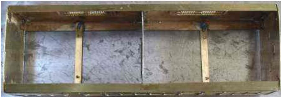
I wanted the body to be removable so two pieces of brass were soldered into the base of the floor and
