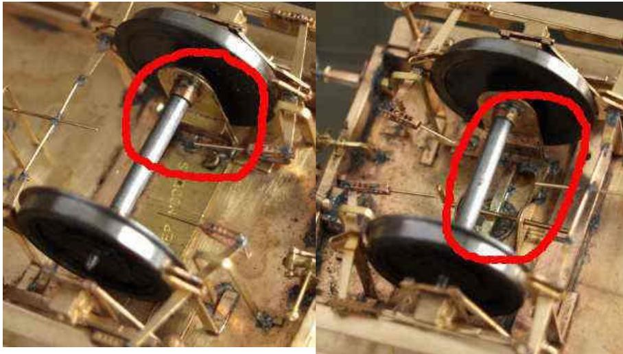
The WEP compensation units were modified to make them more rigid and removable. The rocking unit, on the left, was strengthened to ensure both lateral and vertical rigidity. The 'fixed' unit
