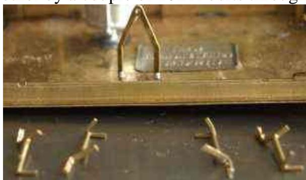
The step board supports are from Slater's and it was necessary to file away a small portion of the lower bulb section to get them to seat properly and shorten the tops slightly. The lower step boards were milled to size from L section and all the edges rounded off.
