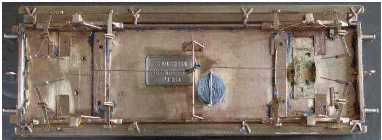
The rodding was then fitted so that the wheels could be removed. The compensation units are from WEP but I have heavily modified them (shewn later) so that they can be removed. One set is held in by its pivot wire and the other by a couple of 10BA bolts through the floor.
