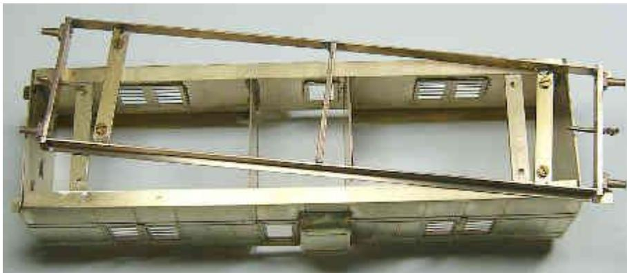
A method of fixing the frame to the body was tackled next. Two pieces of 2mm x 6mm brass strip were cut to fit between the solebars and two more to fit inside the body. One of each was then lined up and clamped together while pilot holes were drilled. The pieces to fit inside the body were drilled and tapped 8BA; other pieces were drilled to clear. The relevant parts were then soldered into the body and across to the frame.
