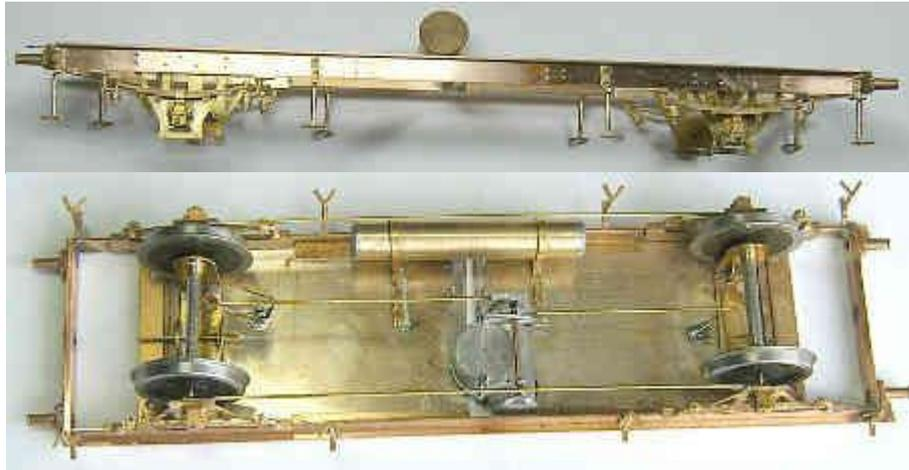
Once the overlays were fitted, eight Slater's footboard supports had the pins cut off and filed nice and flat before being soldered in place. The wheels are to
