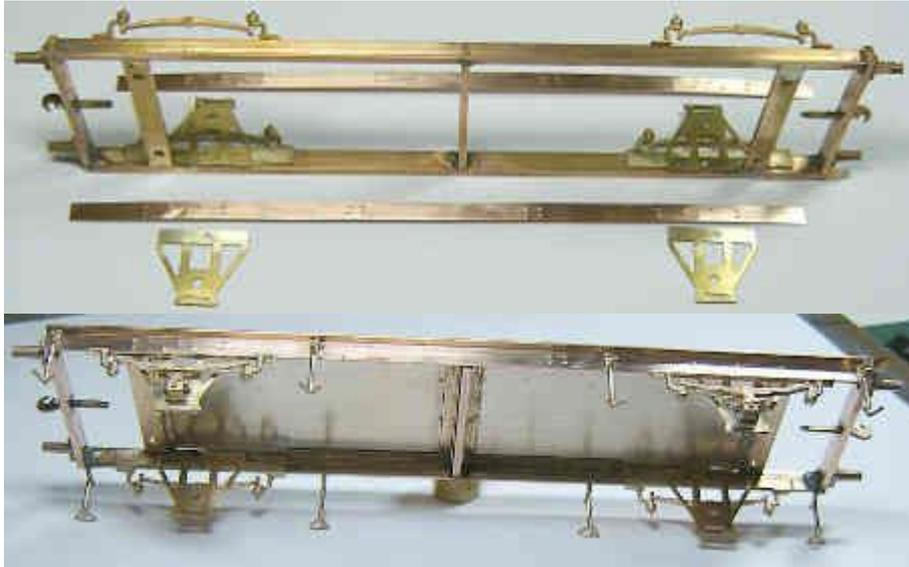
The 18' wheelbase was marked in and a set of CPL lost wax, long J hangers, springs and axle boxes soldered in place. Some W irons from the spares box were soldered in behind them.
