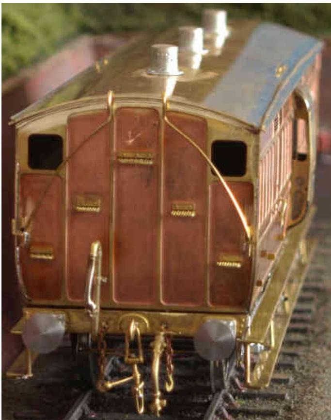
that grab handles would have been fitted to the loading doors by the early 1900s. They are fitted but not fixed yet so they can be removed for painting and are the door handles.
