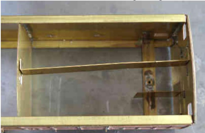
This makes daylight visible right through the side view so I soldered in some scrap brass to act as blinders. Once painted black they should do the job well.
