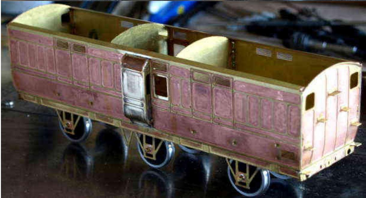
Here the basic running chassis is tested to ensure it is level before further work on adding detail is commenced.
