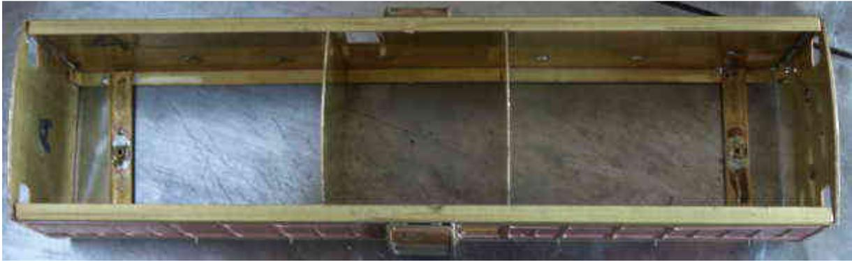
Once the body is soldered up square, the fixing points for fitting the body to the underframe can be fitted. These parts were rather flimsy so I added some rigid U channel to stiffen them up. It is important that the body sits square on the underframe before soldering these parts in place or it will cause distortion and prevent smooth running.
