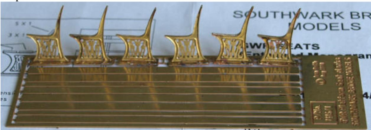
One of the seat planks was lightly marked on the top for centre and 7mm from each end. All the others were simply marked for centre at 81.5mm.
