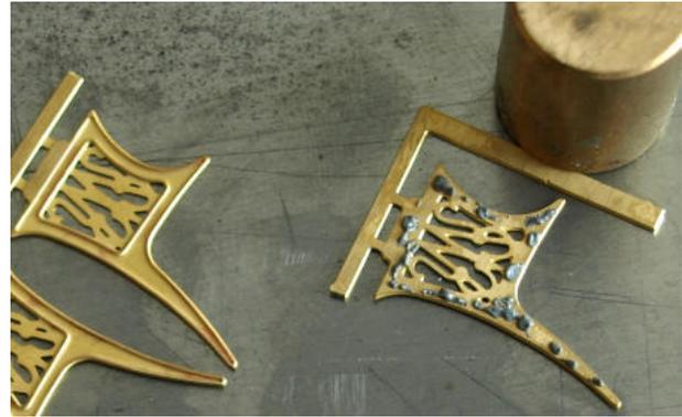
The seat supports are two, mirror image etches so soldering them together is simple. They fit well together. Once soldered together and the cusps all filed off I mounted it in the two parts that makeup the base and soldered it in place. This was done for all the seat supports as
