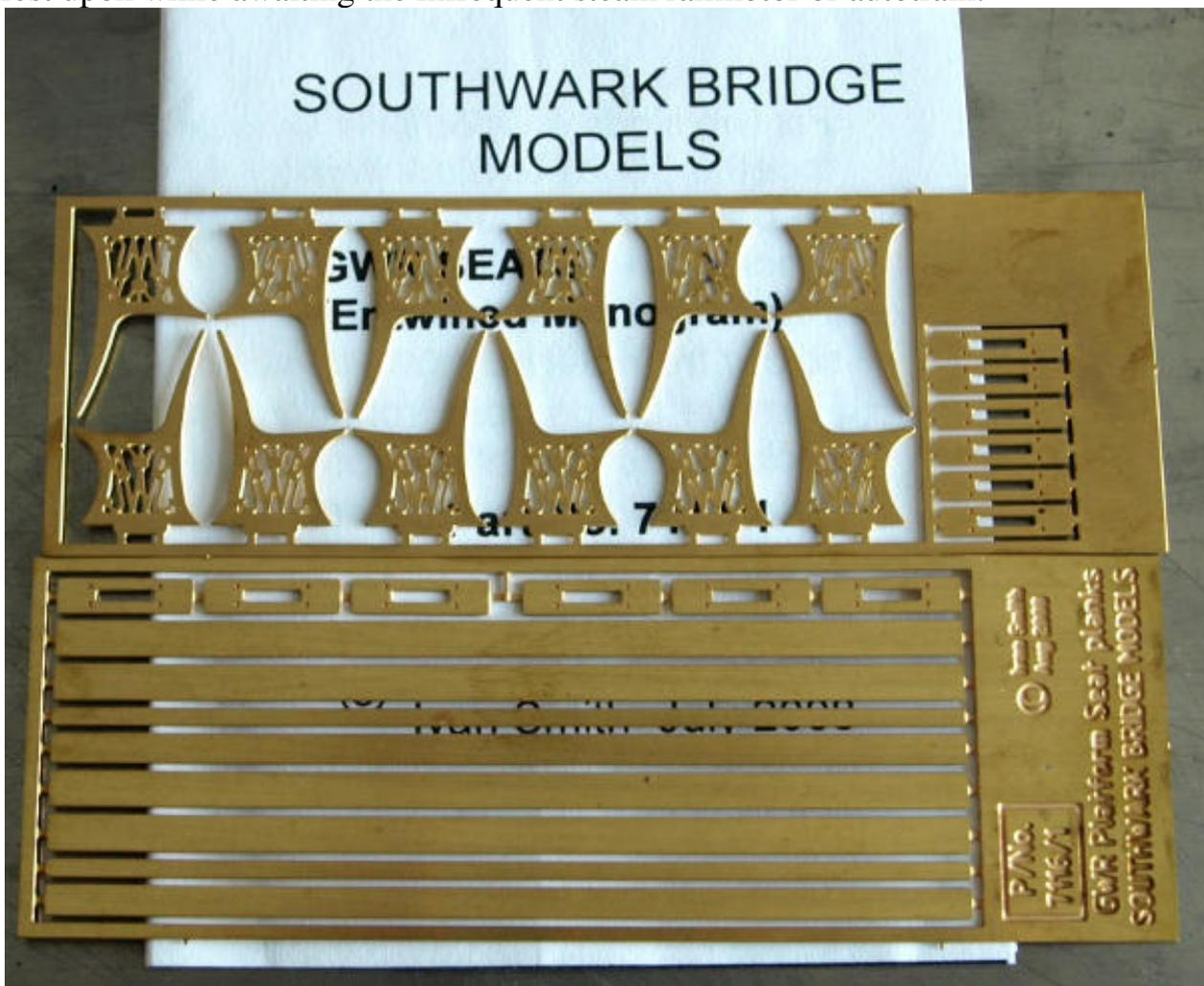
So, what's in the bag? Two small sheets of etch and some simple instructions. The standard of draughtsmanship is, as usual, very high and the etching is excellent too. I was surprised not to find etched dimples in the seat planks to represent the bolt heads but I doubt anyone will notice their lack.
