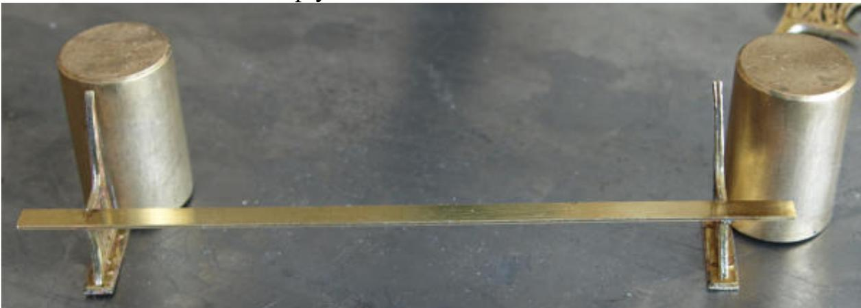
Then, using the trusty magnets to hold two supports, I carefully soldering the first seat plank in place across the outer supports and added the centre one afterwards.
