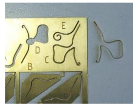
There are a number of jigs provided that makes this item relatively easy. The seat supports are made by bending etched strip in jig C. Here you can see one complete and another in the jig. I found it easiest to start at the end with the tight curl and put the curl in with fine pliers before using the jig. Three identical parts can be produced easily in a few minutes and then soldered up using jig D.
