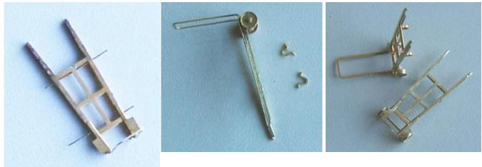
The handholds have been filed to shape and all that remains is to fit the steel "U" supports.
