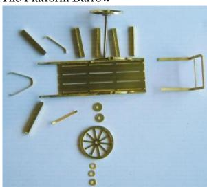
There are quite a lot of parts, here shewn partially completed. The main body is a simple fold-up to which are added another layer for the springs. The instructions suggest making a "back-to-back" gauge for setting the wheels. I did that for the first one and then measured the resulting axle. The other five were made using an axle 21mm long.
