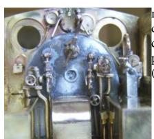
modify odd casting to hand because there were no commercial items available. The cab fittings are a compromise between an excellent picture of the preserved example and the set of parts from Laurie (Shedmaster).
