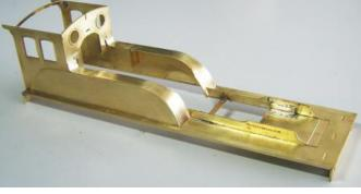
out afterwards. Provided the sides have been assembled correctly, the splasher tops come level with the tops of the splasher sides.
