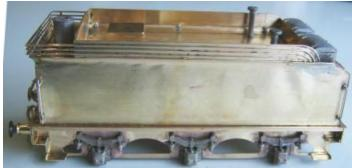
The coal rail etches were used but half round wire (Eileen's Emporium) was carefully soldered over them first. On reflection, it may have been easier to make them from scratch. The chassis was modified to compensate it. Nothing difficult
