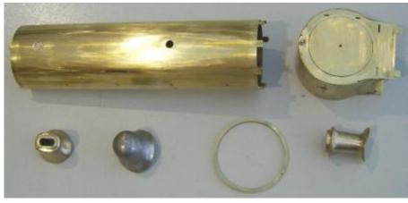
The chimney is a lovely brass casting but the dome and safety valve were very poor and were replaced with better quality items.
