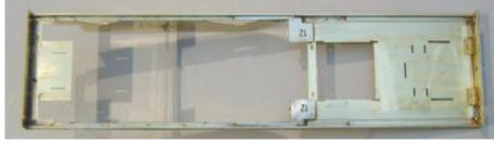
but the front beam is a laminate. I strengthened this too by adding some angle as you can see from this picture.
